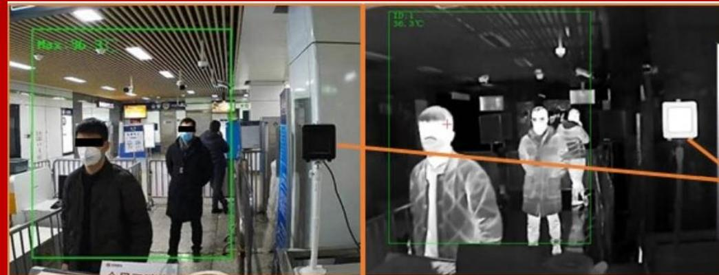
\*Enhanced with a blackbody calibrator to increase the temperature measurement accuracy from **0.5°C to 0.3°C.**
